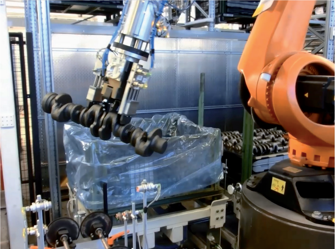
Roboter greift Kurbelwelle aus Gitterbox / Robot picks up crankshaft from a pallet cage.
